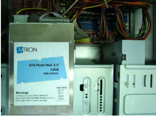
Figure 3: MSD-P35 NAND Flash-based Solid State Disk
